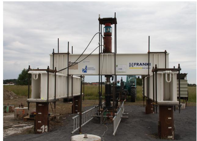
Figure 3: Two-way pile load test set up at Merville
